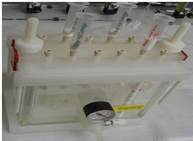
Figure 4. Visiprep Solid Phase Extraction Vacuum Manifold
