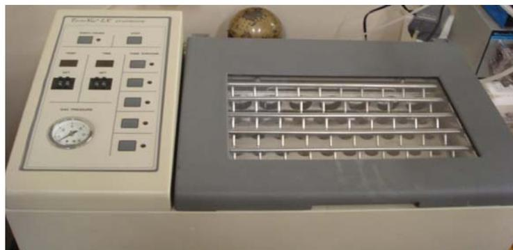
Figure 5. TurboVap LV evaporator
